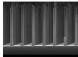
Array of nanowires gallium phosphide made with an electron microscope. Photo: Eindhoven University of Technology.
