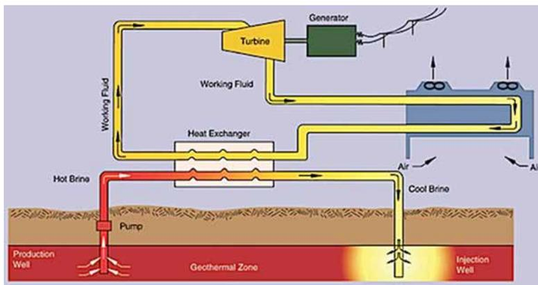
Figure 1. Schematic diagram of a geothermal power plant (credit [www.seg.gov](http://www.seg.gov)).
