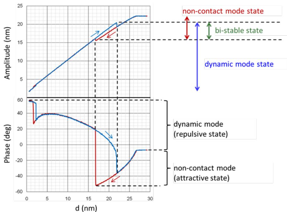
Figure 1. AFM cantilever oscillation amplitude (upper) and phase (lower) vs. tip-sample separation ( $d$ ) known as the A-d curve for constant  $Z$  actuator driving power. The red curves denote the tip approaching the sample and the blue curves show the response when the tip is retracted from the sample surface. (Image used with permission from Nanoscientific)[7]
