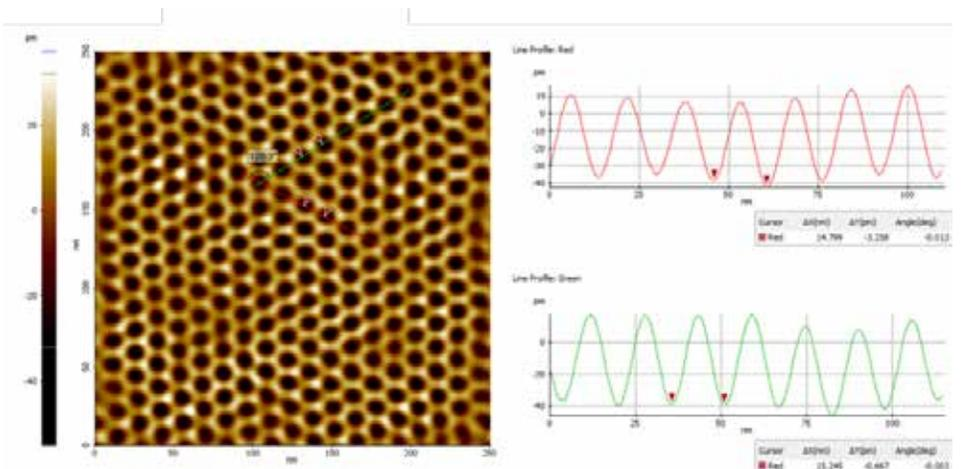
Figure 4. A FFT filter is applied to one of the 250nm images in Fig. 2.a. to characterize the moiré superlattice. Line profiles for the red and green lines are shown on the right side.
