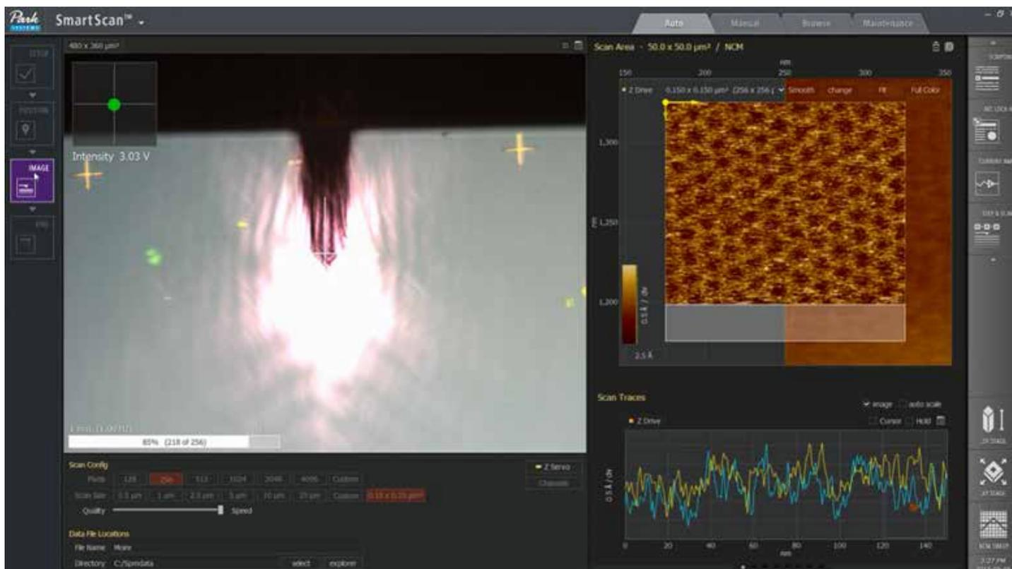
**Figure 2.** The newly developed SmartScan™ Auto Mode which allows automated sample surface detection and imaging with minimal user interaction. On the left the major buttons including “positioning” and “image” are shown. Screenshot was taken while the software was collecting a 150 nm image of graphene/hBN sample in Non-Contact mode. User only needs to select scan size, image resolution, and quality/speed.
