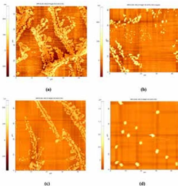
Figure 3. AFM images of the silica polymerized from (a) untreated geothermal fluid, (b) 5.0 ppm, (c) 8 ppm, (d) 10 ppm of phosphinocarboxylic acid.
