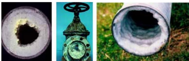
Figure 2. Scaling and Silica deposition on pipes handling geothermal brine (credit [www.geokem.co.nz](http://www.geokem.co.nz))
