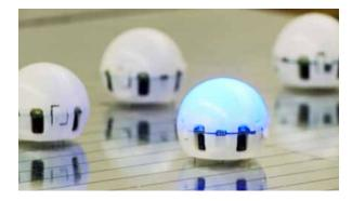
Researchers at University of Colorado have built a swarm of 20 robots, each robot being about the size of a pingpong ball. Possible future use for such teams of intelligent robots could be tackling a number of challenging situations, from containing oil spills to self-assembling into large installations of hardware after being launched into space or deployed deep under the ocean.
