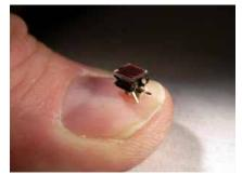
Solar Micro bot- tine robots used for data collection
